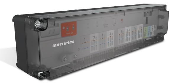
The 22-00013 has 8 control zones, each with connections for up to 3 heating zones (actuators). The pump logic and boilers logic, a connection for Dew point sensor and the C/O input for automatic switching from heating to cooling are standard.
