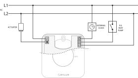
The jumpers from 1 to 5 are representing the number of actuators that you can connect to the thermostat.
