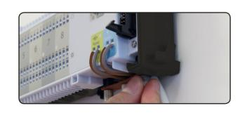
Make sure the fuse is fitted (4Amp).
