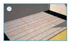
Upon completion of the first row. start the process again by placing two more End Supports next to the existing ones, and secure with the integral inter-locking points.
