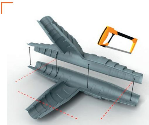
**ENG** Cut the shells of the insulation set according to the desired jacket pipe diameter. The shell with the groove is used as bottom shell.
