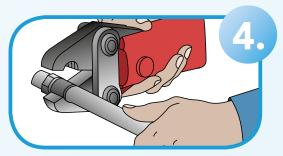
Position the press tool jaws between the double guides on the sleeve and press the fitting. Close jaws and start pressing procedure.
