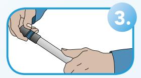
Slide the fitting onto the pipe until it appears in the inspection window.
