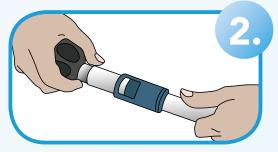
Calibrate the pipe using the correct bevelling tool.
