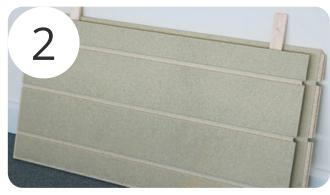
Before installation, separate the boards with battens and place them close to the conditions of use. The boards should be left in the room of application for five days before laying. This will acclimatise the moisture content of the Fortis Timber boards should be acclimatised close to the conditions of use.
