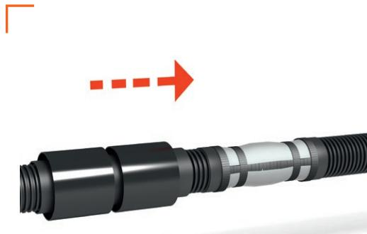
**ENG** Slide over the straight covering jacket pipe, until both ends of the pre-insulated pipe are covered. Then slide over both shrinking sleeves, each of them covering half straight covering pipe and half jacket pipe.
