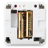
turn over and pull out the old batteries. Replace with fresh Alkaline batteries (do not use zinc or rechargeable batteries)
