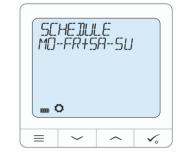
using  $\sim$  scroll through the different programme types, press  $\checkmark$  when happy
