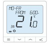
next set the temperature using the then press to accept and moe to next interval
