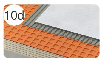
If the tiler wishes to install a decoupling membrane between the UFH boards and tiles, we recommend following the procedure in 11a with Mapei Keraquick S1 then fixing the mat down onto the adhesive bed. Once cured, the tiling can commence to the tilers normal regeme. But please ensure any adhesives used are suitable for UFH systems.
