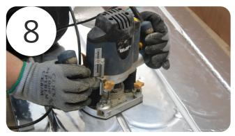
If you have to alter the panels, we recommend using a knife or a router to channel a new route.
